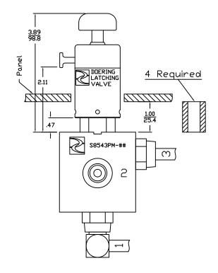
Panel Mount housings may be mounted directly to the site panel, or Doering SD- Series Stand Off Spacers may be used to improove access to the valve wrench hex area or to control the protrusion of the valve from the panel face. Please see Doering SO- Series Stand Off Spacers on Spec. Sheet 1203290.
