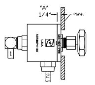
Example using: \$85#2PM-## Housing, Panel Mount \$85-025-PM# Spacer, Panel Mount, 0.25" Doering Needle Valve
