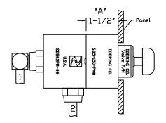
Example using: \$85#2PM-## Housing, Panel Mount \$85-150-PM# Spacer, Panel Mount, 1.50" Doering Manually Operated Valve
